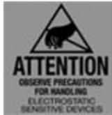
As with all electronic devices, they are susceptible to damage by static electricity discharge. Before removing the cover of this product be sure to discharge the static electricity in your body by touching a piece of grounded metal.
